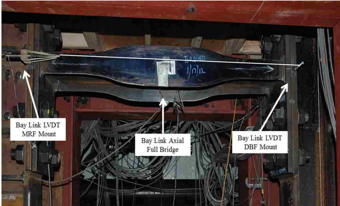
Figure 5.5 – Bay Link Instrumentation
